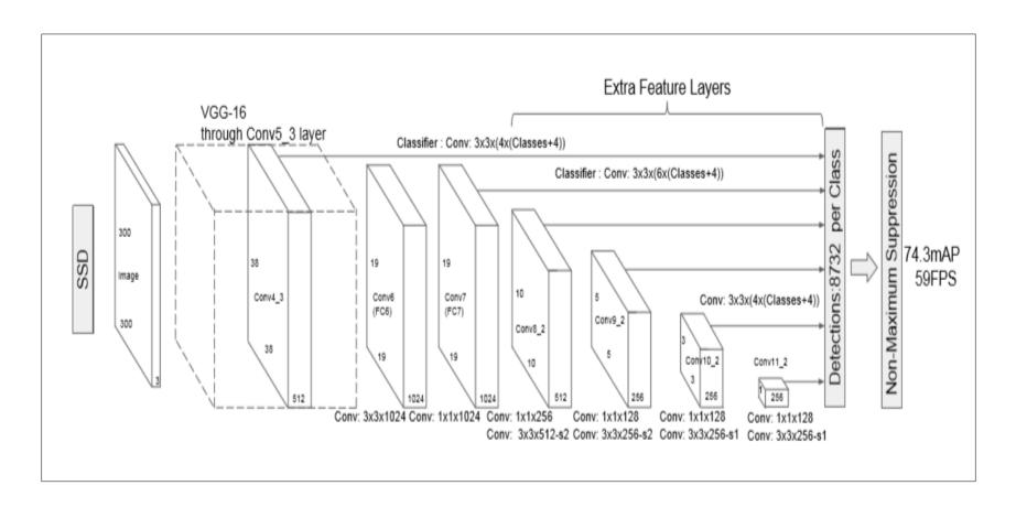
**Architecture of SSD compared to YOLO**: It adds several feature layers to the end of a base network, which predict the offsets to default boxes of different scales and aspect ratios and their associated confidences. SSD with a 300×300 input size significantly outperforms its 448×448 YOLO counterpart in accuracy on VOC2007 test while also improving the speed.
