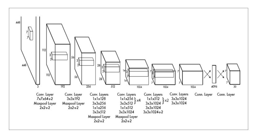
**The Architecture :** Our detection network has 24 convolutional layers followed by 2 fully connected layers. Alternating  $1\times1$  convolutional layers reduce the features space from preceding layers. We pretrain the convolutional layers on the ImageNet classification task at half the resolution ( $224\times224$  input image) and then double the resolution for detection.
